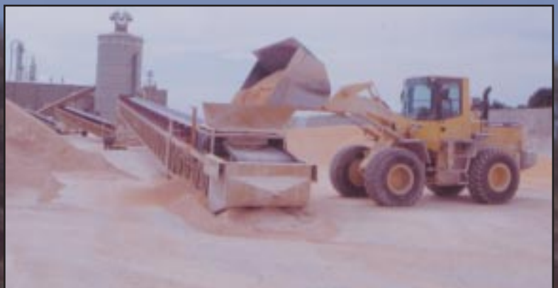
Corn is loaded onto a conveyor belt that feeds the new ethanol plant at Sioux Center.
