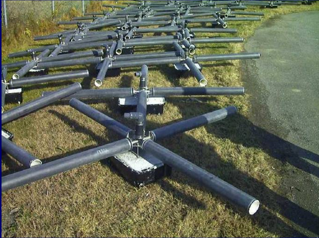
Caribou aeration units
