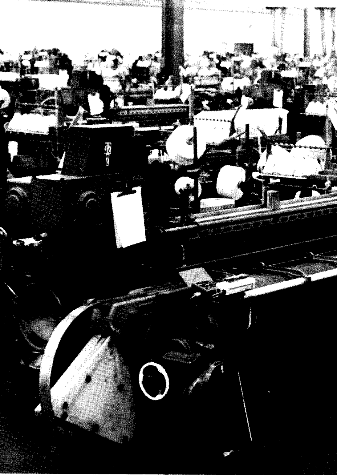
Open-end spinning weaves cotton fibers into denim in American Cotton Growers Littlefield, TX, plant. Inset, denim fabric is being wrapped for shipment.
