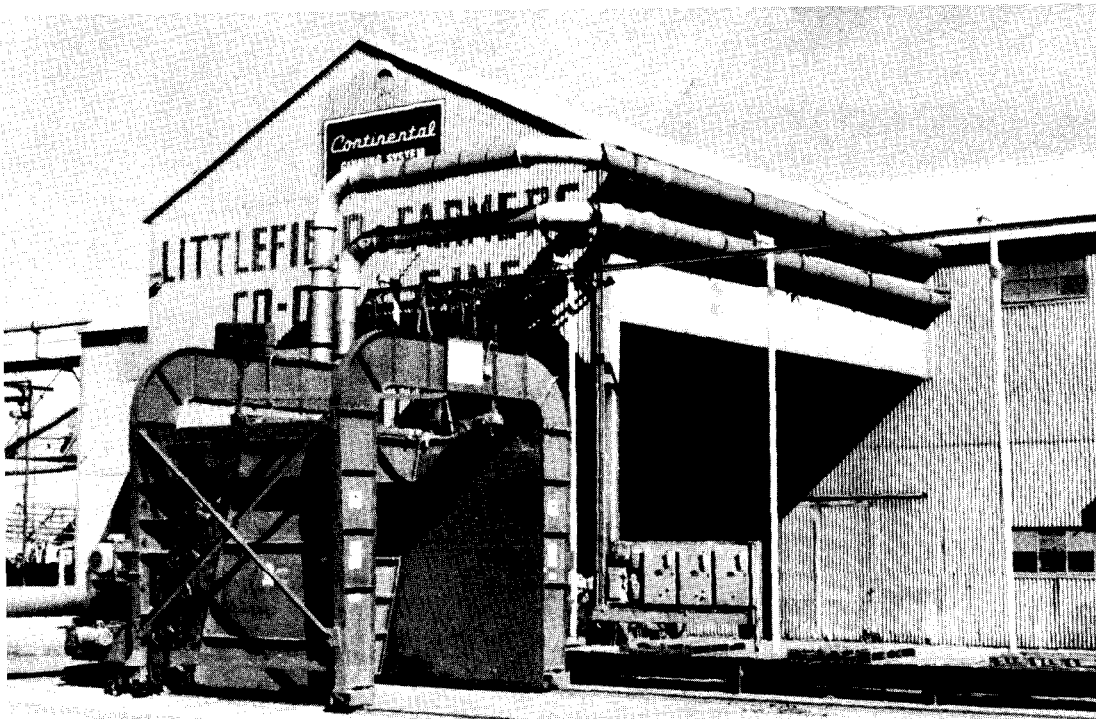
Littlefield (TX) Farmers Cooperative Gins has modernized with an automated handling system for receiving seed cotton. Inside the gin, seed is separated from the lint.
